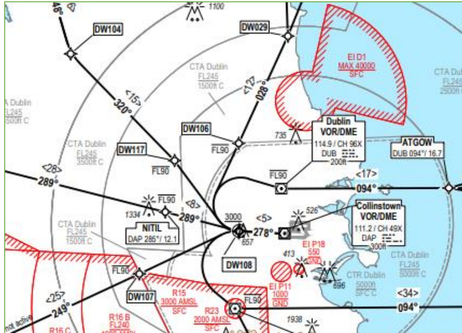
SID for South Runway (28L) Departures to the west (Westerly operations in westerly winds)
